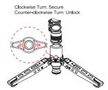
4.2 Loosen the Ball Locking Knob to tilt the monopod  $36^{\circ}$  in any direction.
